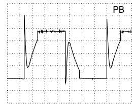
DC, 2V/Div, 1ms/Div Connector 1930-(1), -(2), -(3) ⑤⑥
